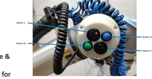
Hardware & software interface for robot programming by manual guidance
