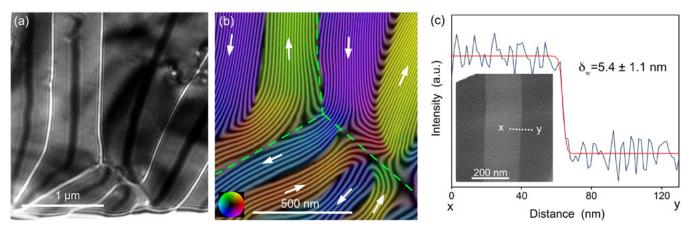
Fig 1.: Magnetic imaging studies of the grain-boundary diffusion processed Nd-Fe-B magnet
