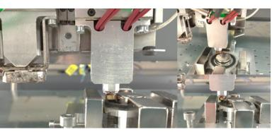
Fig 6: Printing of ring-shaped magnets
