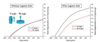
Fig 5: Magnetic properties of ring-shaped magnets with and without external magnetic field
