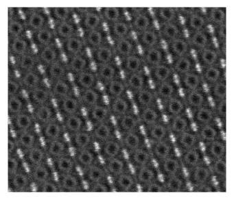
Fig. 3: Atomic resolution Z-contrast image of a  $Nd_2Fe_{14}B$  crystal grain viewed in the [100] zone axis
