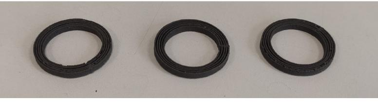
Fig 8: Ring-shaped magnets
