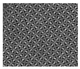
Fig. 2: Atomic resolution Z-contrast image of a  $Nd_2Fe_{14}B$  crystal grain viewed in the [001] zone axis
