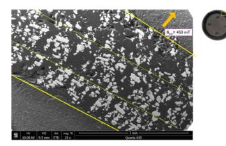
Fig 7: Particle Alignment due to the external magnetic field during printing process
