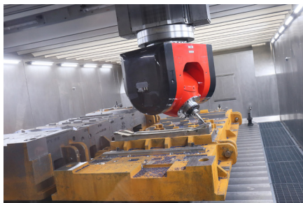
Rezkanje odlitka – Milling of the casting
