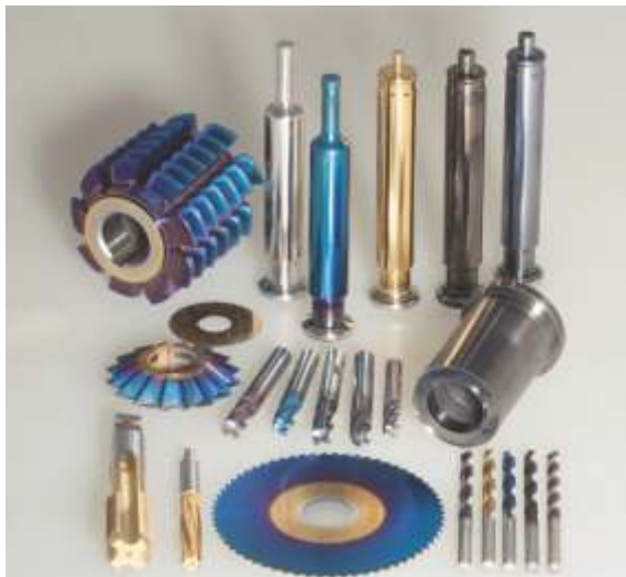
Kolekcija rezalnih in preoblikovalnih orodij, prekritih z različnimi trdimi prevlekami A collection of cutting and forming tools protected by various hard coatings
